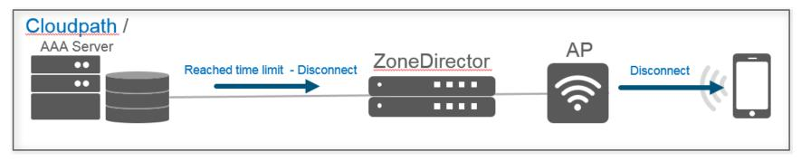
1. Simplified yet dynamic control of users' access to WLANs. As the above diagram illustrates, a user has paid to access a WLAN for internet connectivity. Upon reaching the time limit, the radius server pushes a CoA message to disconnect the user from the network. Other supported CoA attributes can be leverage to enforce certain actions dynamically.
